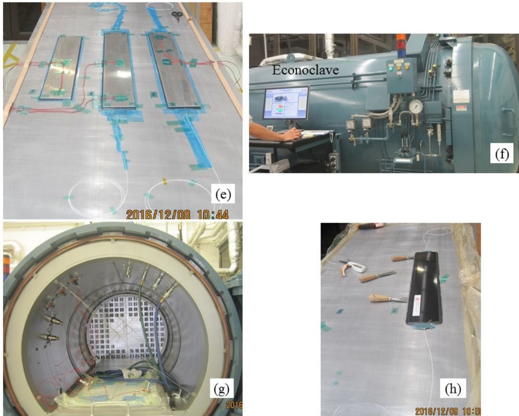
Fig. 4 Fabrication procedure of the smart CFRP-FBG composite: (a) FBGs in series fixed on the 8-layer CFRP strips; (b) 16-layer CFRP strips embedded with FBGs in series; (c) Seal for vacuum preloading; (d) Initial molding composite; (e) Installation of thermal couplers; (f) ASC process system; (g) Second molding composite; (h) CFRP-FBG composite
