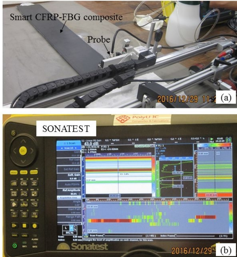
Fig. 7 Ultrasonic testing on the CFRP-FBG composite: (a) Ultrasonic probe; (b) Flaw detector
