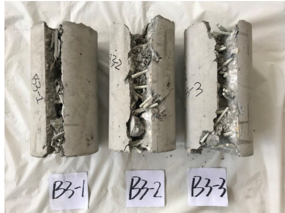
(b) Cylinders with GFRP needles
