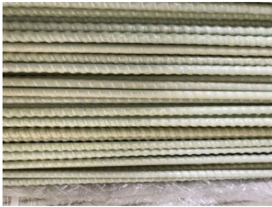
(c) Helically wrapped rebars
