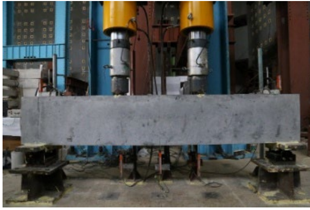
Figure 12. Test set-up of the large-scale RC beam specimens
