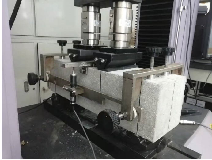
Figure 5. Setup of flexural tests.
