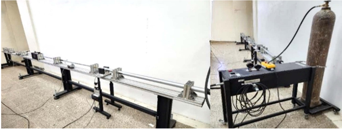
Figure 5. Two views of the SHPB device installed at Hakim Sabzevari University.
