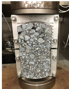
Figure 2. Specimen for overlay tests.
