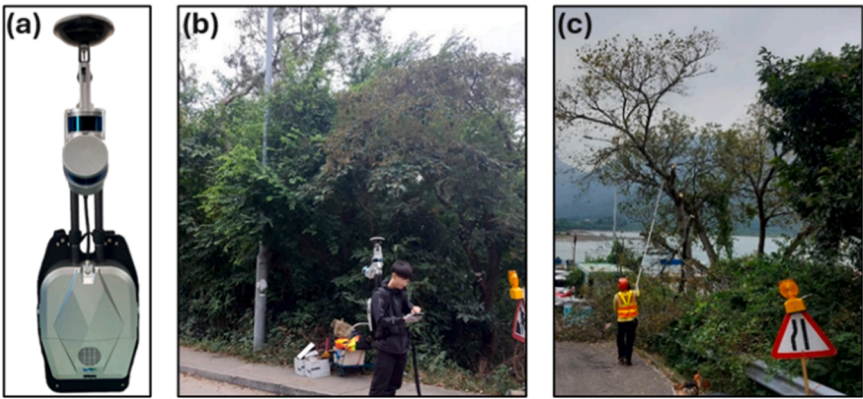
Fig. 3. (a). LiDAR backpack; (b). LiDAR backpack survey; (c). Tree felling practice.
