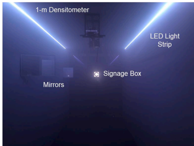
Fig. 3. (a) New experimental setup for signage visibility experiment: (b) front view of the chamber and (c) back view of the chamber.
