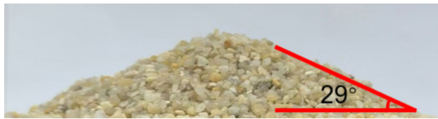
Fig. 12 Column collapse test of sand
