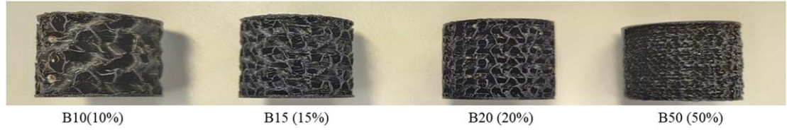
Figure 10. 3D printed materials with different infill densities.
