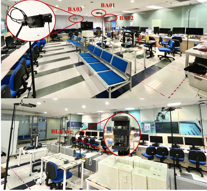
Fig. 4. The deployment of BLE indoor positioning system.
