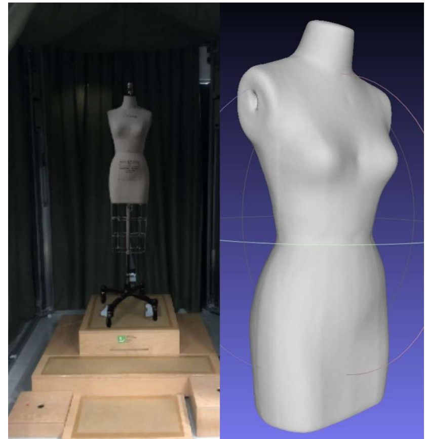
Figure 6. A size 10 dummy in a body scanner TC2 and a virtual model of size 10 dummy.
