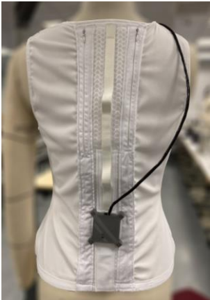
Vibrotactile Feedback (VTF) system with IMU sensors for postural monitoring
