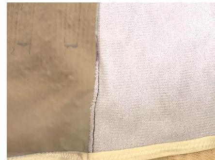
Pilling on tricot fabric of the original design
