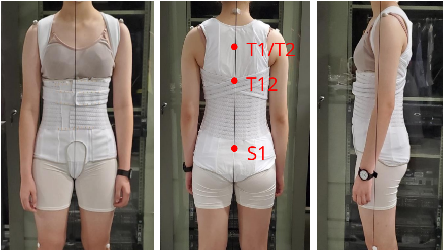
Front, back, and side views of the posture correction girdle on a subject, showcasing IMU sensors (indicated by red dots) installed along the spine.
