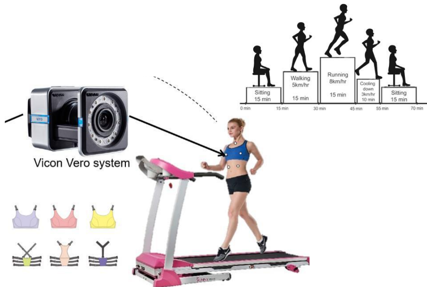
Motion measurements of the human body and breasts under 30 bra conditions at various running speeds
