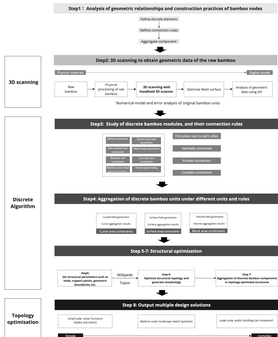
Figure 11. Digital workflow of steps: from scanning to discrete to topological.
