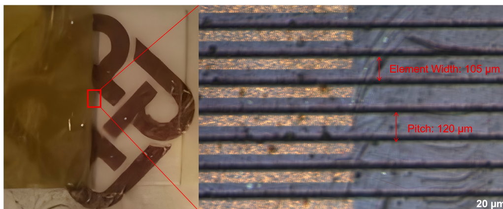
Fig. 2. Photograph of developed TUT array.
