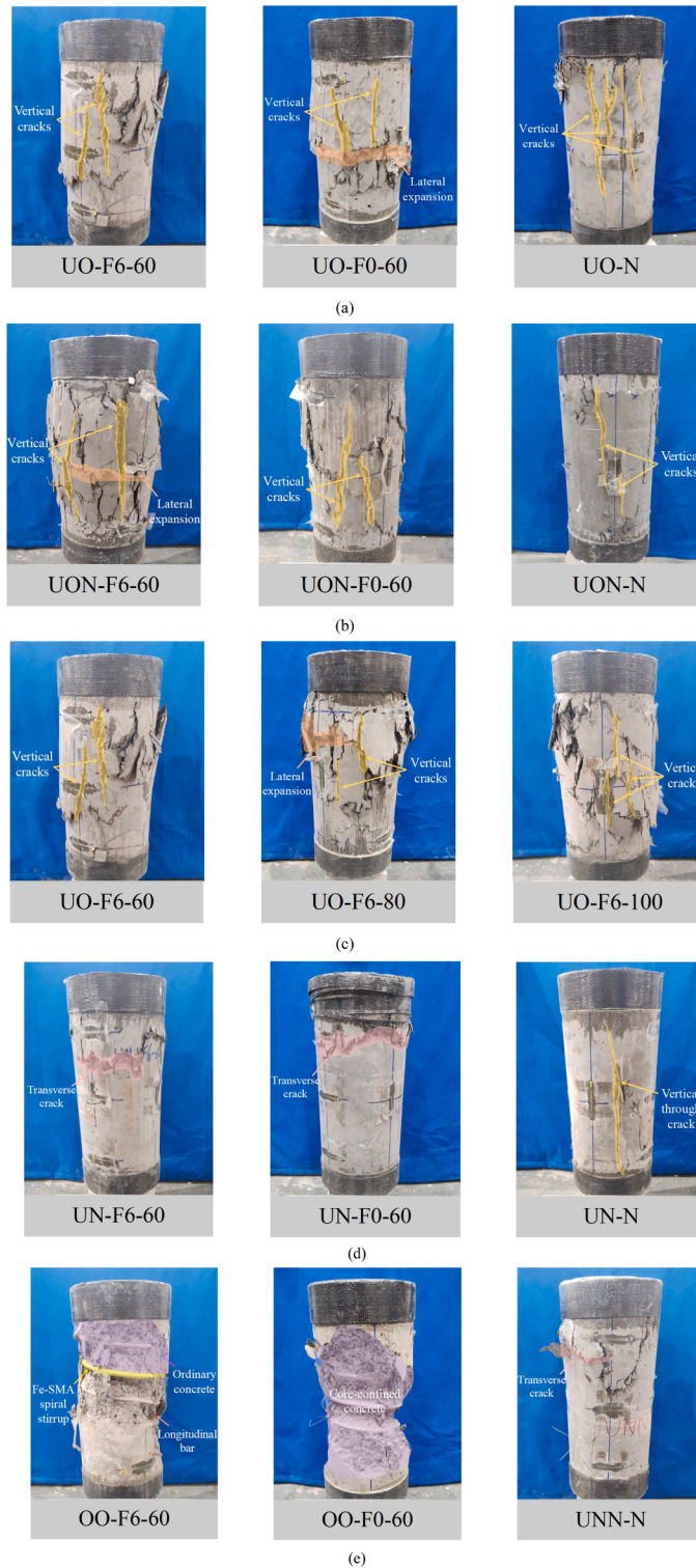
Fig. 7. Failure modes of specimens: (a) composite columns after autoclave curing; (b) composite columns after natural curing; (c) composite columns with varying stirrup spacing; (d) UHPC tubes after autoclave curing; (e) ordinary concrete columns and UHPC tube after natural curing.
