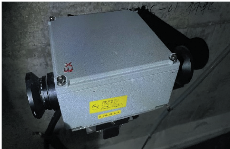
Figure 2. The inertial camera instrument is set up inside the bridge.
