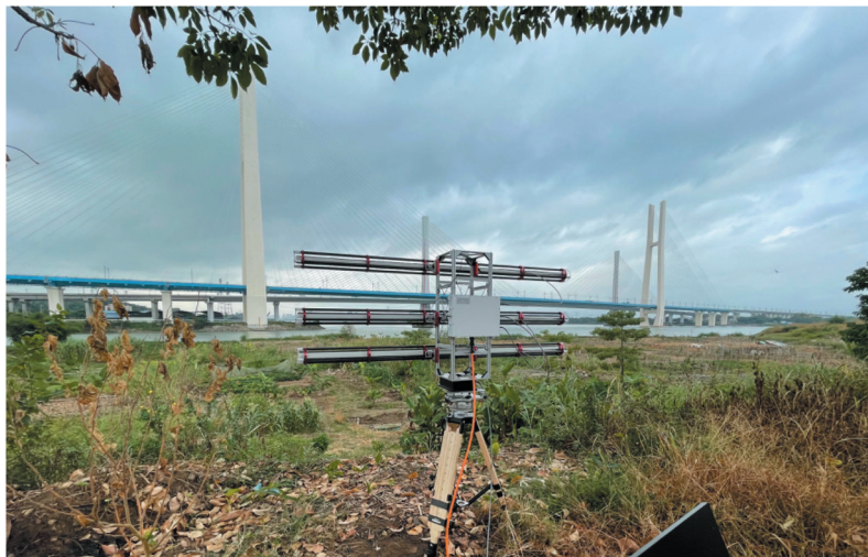
Figure 1. The GAMMA GPRI II instrument.
