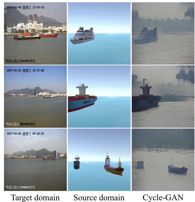
FIGURE 12 Cycle-consistent generative adversarial network (Cycle-GAN) model-based image transition.
