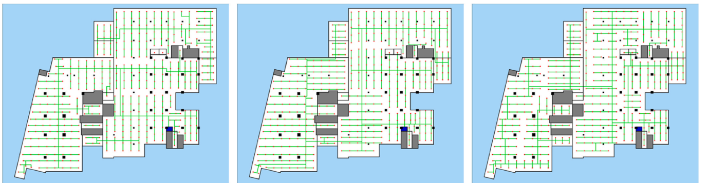
Fig. 9. Examples of different pipeline connections for the same sprinkler placement.
