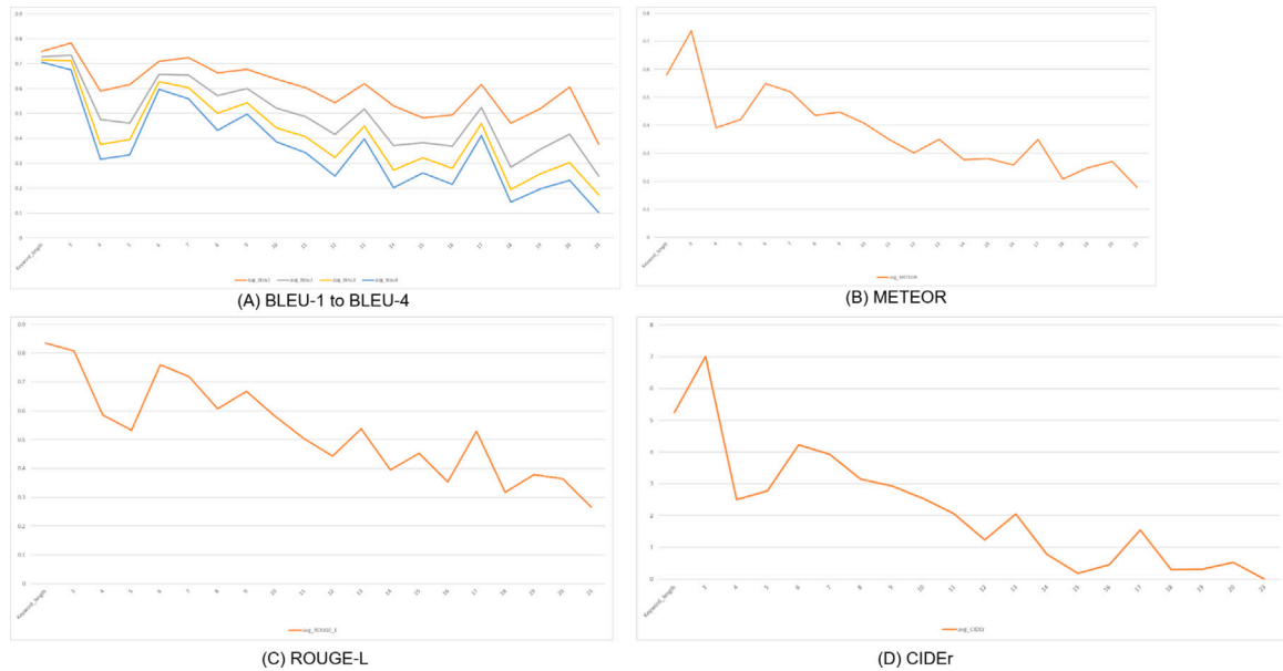
Fig. 13. Performance and keyword list length distribution in the IU X-ray dataset. This figure illustrates the relationship between keyword list length and the performance of the proposed method on the IU X-ray dataset. The results show a general decline in performance across all evaluation metrics as the keyword list length increases. This trend suggests that longer keyword lists correspond to more complex radiology reports, which pose greater challenges for accurate generation. The analysis highlights the difficulty of handling lengthy and detailed inputs, emphasizing an area for future improvement in radiology report generation models.
