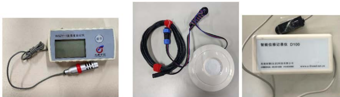
(a) Temperature and humidity self-recording logger (b) PIR sensor (c) Intelligent displacement recorder
