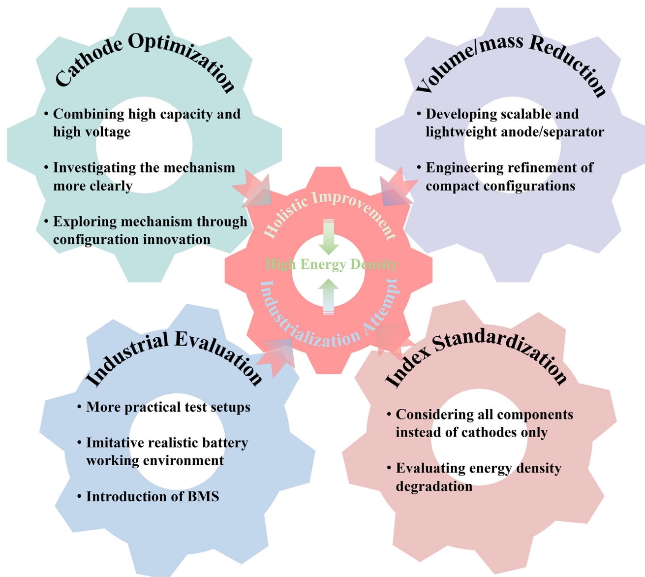
Figure 18. Perspectives of strategies to design high energy density aqueous zinc-ion batteries.
