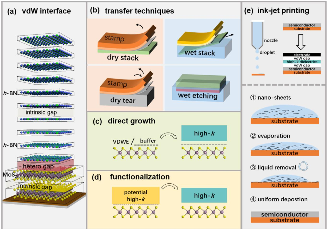
**Figure 2.** Schematic of integration methods for vdW interfaces. (a) A typical vdW interface formed by multilayer  $h$ -BN and monolayer  $\text{MoS}_2$ . (b) Top-down transfer methods. (c)-(d) Bottom-up methods. (e) Ink-jet method diagram.
