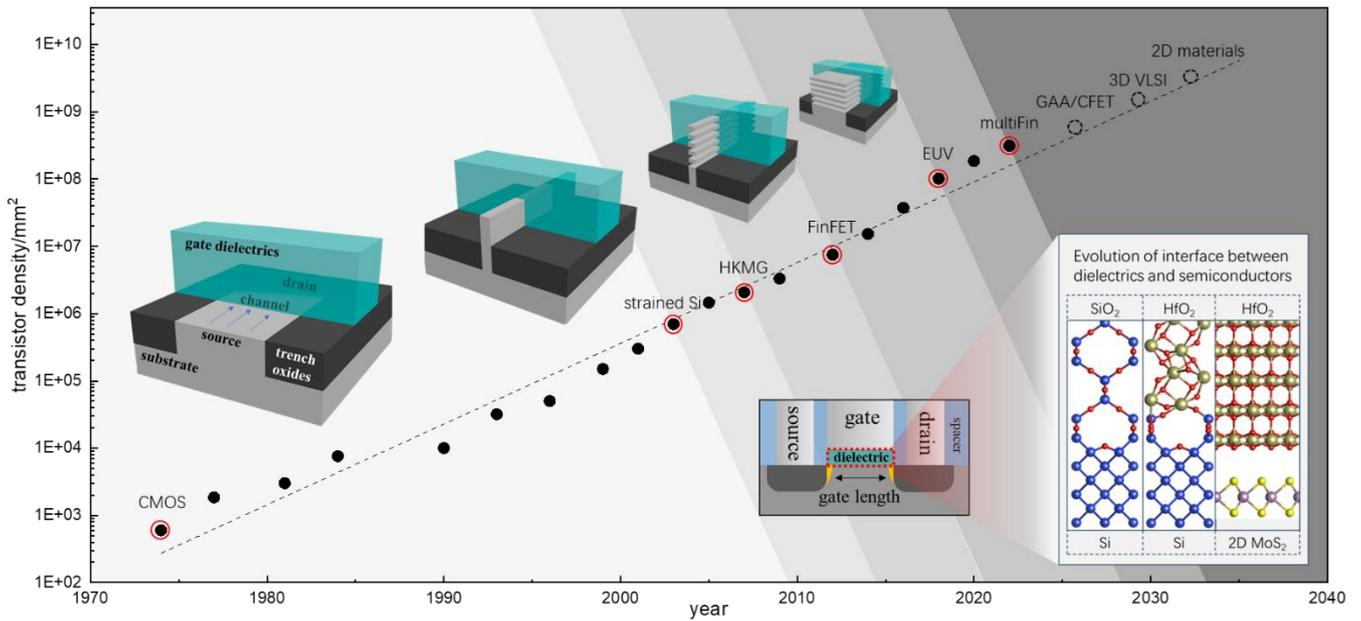
**Figure 1.** Trends in transistor miniaturization over time. The main technology nodes of transistor are shown with time evolution. Four geometries of transistors are depicted with size scaling. The inset shows representative semiconductor-insulator interfaces.
