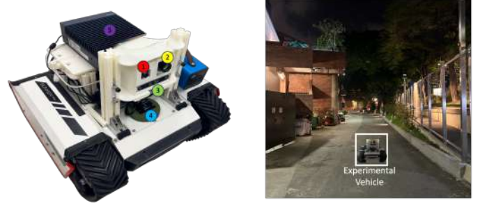
Fig. 9. Experimental vehicle system(left) : (1) Dvexplorer mini, (2) Optris 450PI, (3) Realsense D455, (4) CMP10A, (5) Intel i5-12400 CPU computer and environment (right).
