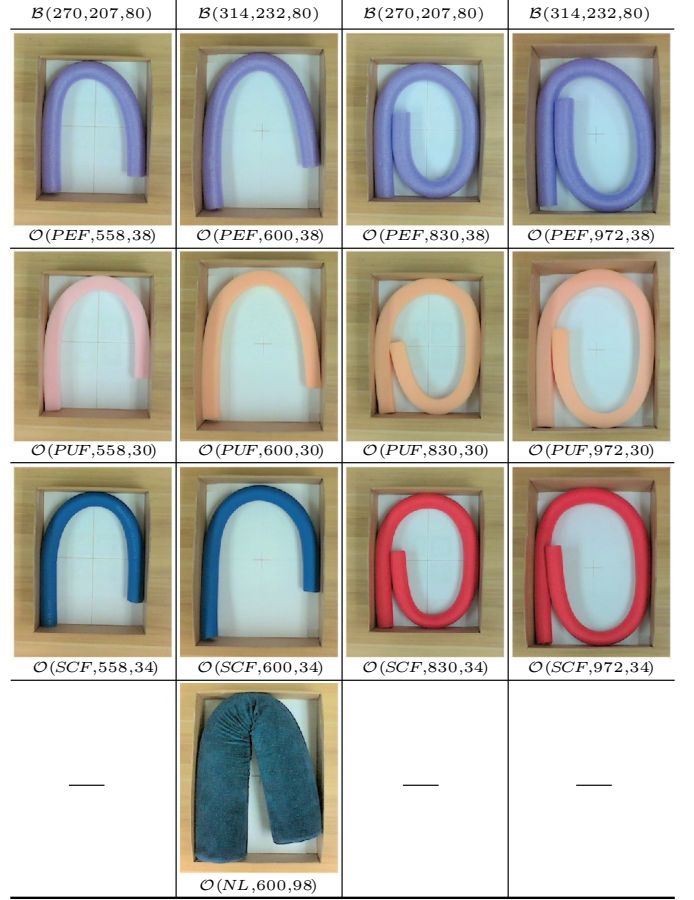
Fig. 9. Packing 13 objects \mathcal{O}(\eta, l_O, d_O) of different lengths into two boxes. PEF: Polyethylene Foam, PUF: Polyurethane Foam, SCF: Silicone Foam, NL: Natural Latex.
