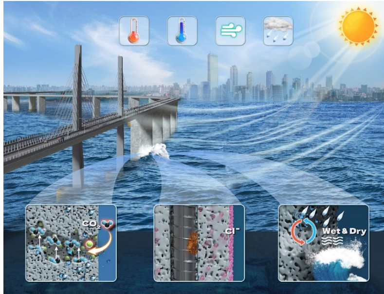
Fig. 1. Schematic of different exposure zones in a coastal RC structure and the critical micro-climate factors affecting chloride transport and chloride threshold in each zone
