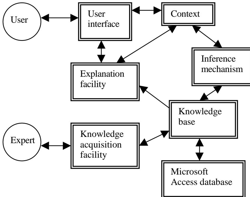
Figure 2. Schematic view of the expert system.
