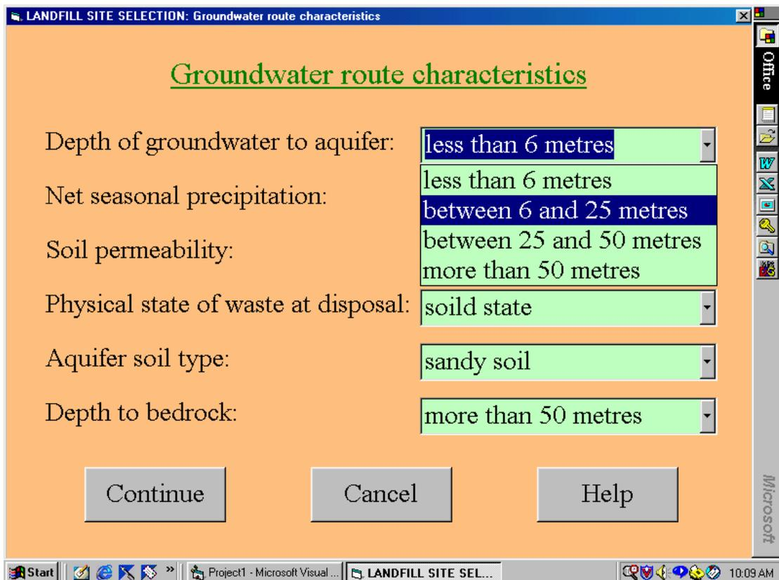
Figure 3. Screen displaying user-friendly data input of groundwater route characteristics.
