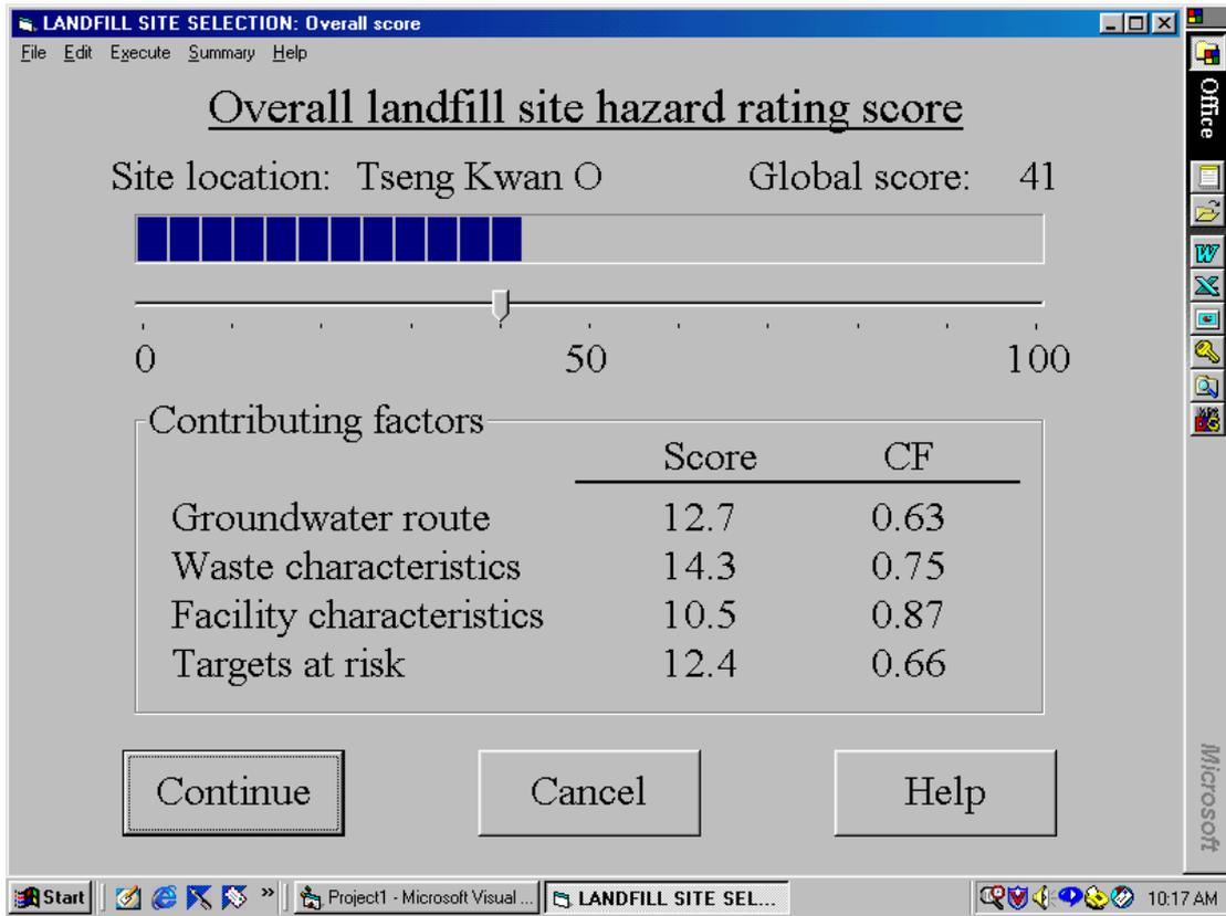
Figure 4. Screen displaying overall landfill site hazard rating score.
