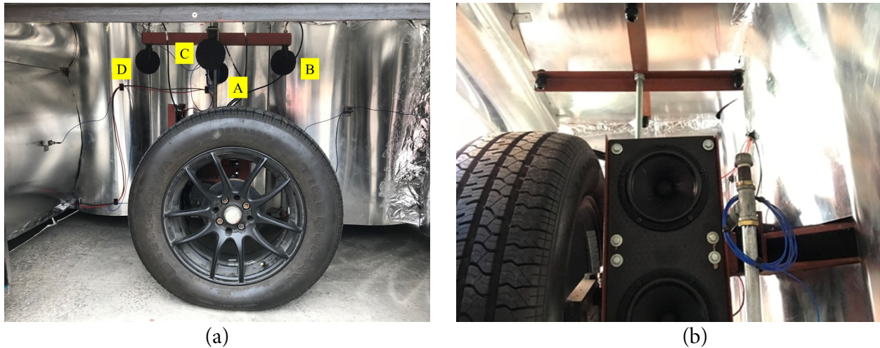
Figure 2: Microphones and RSS setting in the reverberant chamber.
