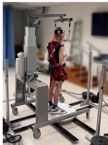
Figure 1. The moving-platform perturbation system being used by a participant.
