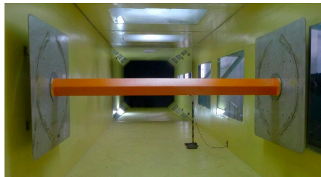
Figure 4. Section model suspended in wind tunnel.
