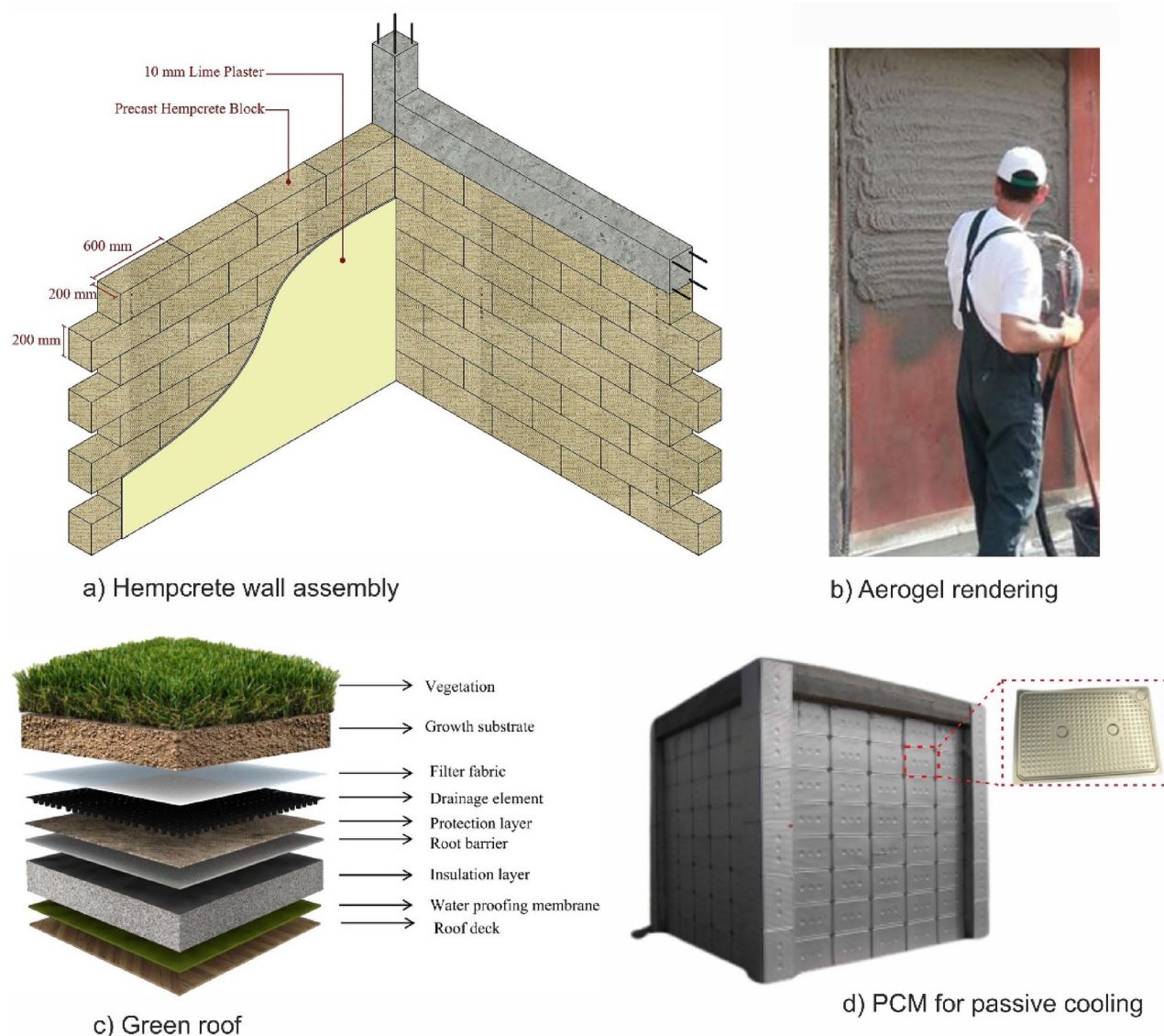
Fig. 3 Various alternative materials in building construction a Hempcrete [87]; b aerogel rendering [88]; c green roof [89]; d phase changing materials (PCM) [84]
