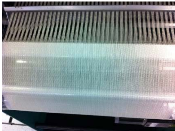
Fig. 3. Integration of optical fibers into fabric, processed on a weaving loom
