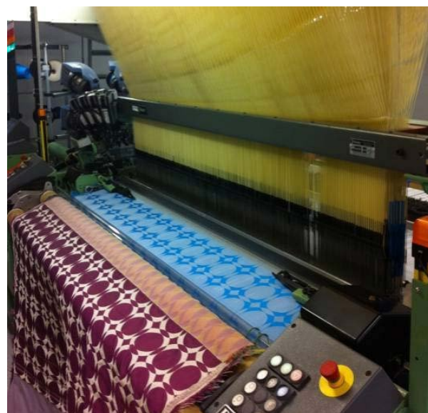
Fig. 8. Optical fiber integrated fabric that is being processed on a weaving jacquard loom
