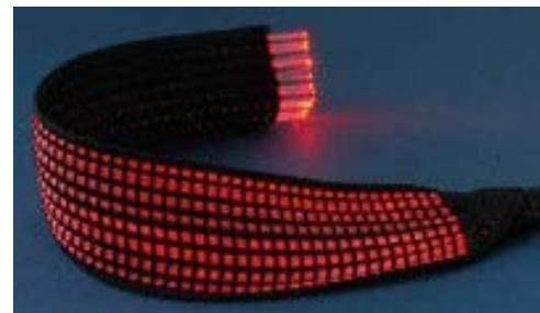
Fig. 3. Optical fibres woven into belt
