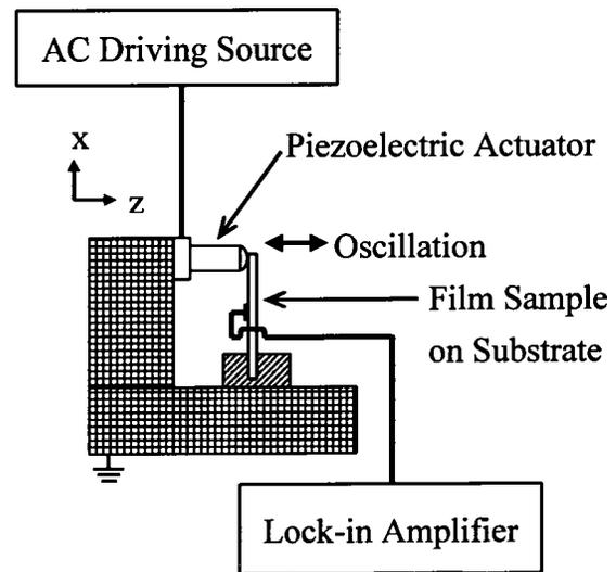
FIG. 1. Experimental setup for the measurement of the transverse piezoelectric charge coefficient  $e_{31}$ .
