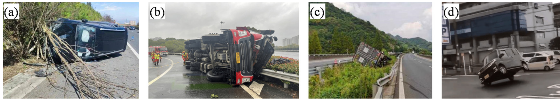
FIG. 1. Traffic accidents caused by crosswinds: (a) rollover, Hang-Rui Expressway, Yunnan, China, 2022; (b) rollover, Hu-Ning Expressway, Jiangsu, China, 2022; (c) rollover, Yong-Jin Expressway, Zhejiang, China, 2020; and (d) lane departure, Tokyo, Japan, 2021.
