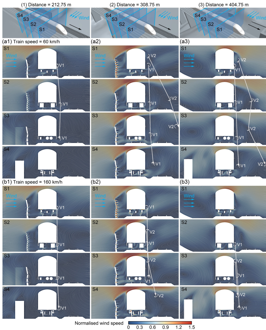
FIG. 20. Normalized wind speeds and streamlines around leading vehicle at different locations along railway line at different train speeds of: (a) 60 and (b) 160 km/h. (Inlet wind speed is at 30 m/s.)
