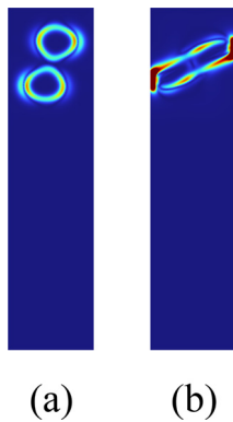
FIG. 7. Distribution of force of the case with flat walls at V_0 = 2000 V for different moments: (a) t = 0.01 s; (b) t = 0.05 s.
