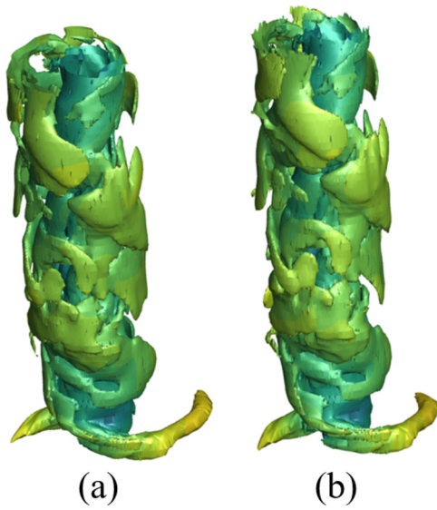
FIG. 17. Comparison of the instantaneous vortex structures ( Q = 1.8 \times 10^5 \text{ s}^{-2} ) colored by pressure between the (a) real result and (b) predict result.
