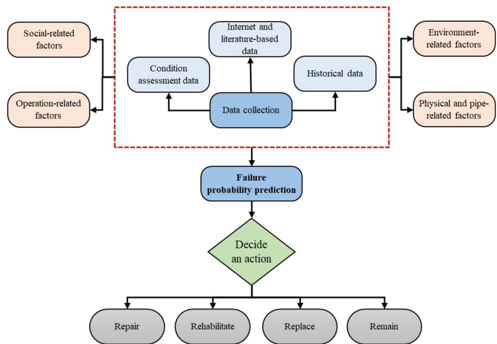
**Figure 1.** Conceptual framework for decision-making process regarding failure probability of water pipes.
