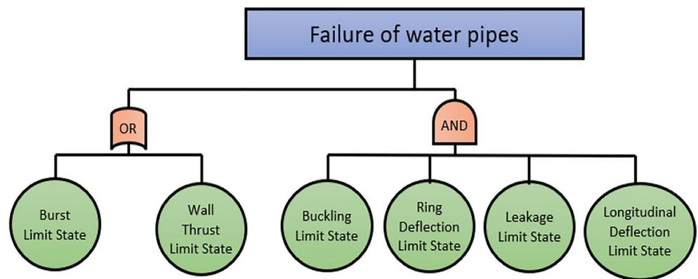
Figure 7. Multiple failure modes.
