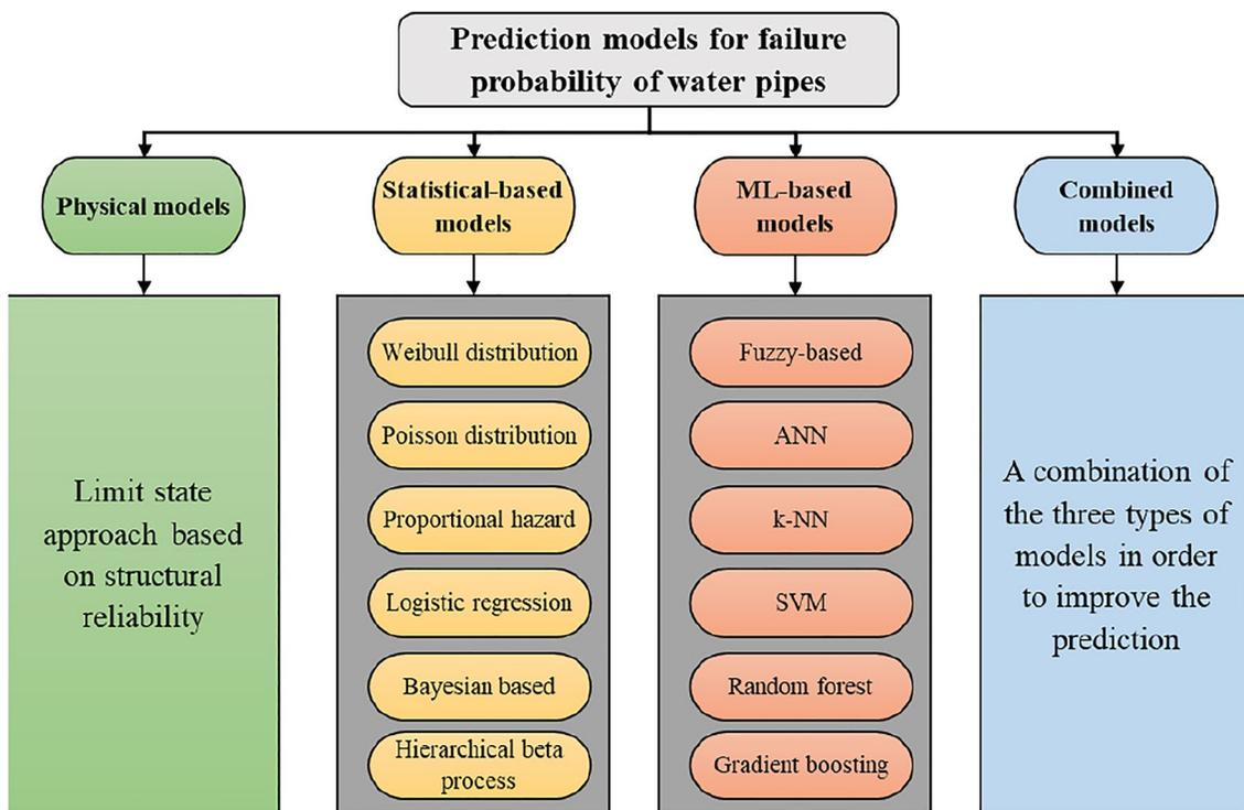
Figure 6. Prediction models for failure probability of water pipes.
