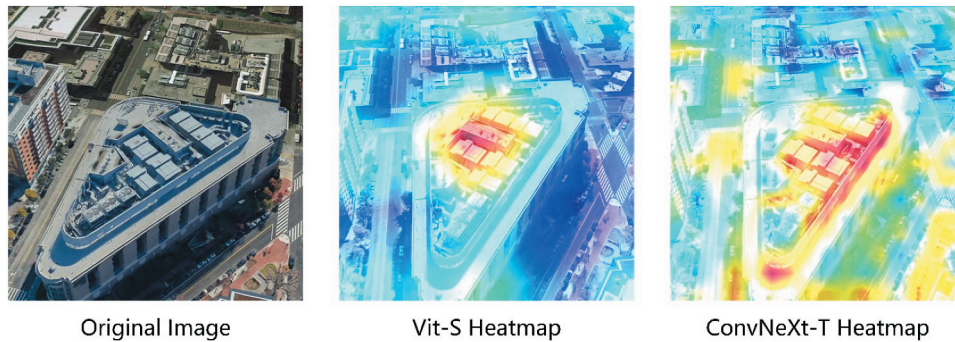
Figure 4. The ConvNeXt network and backbone network heatmaps. The initial picture is on the left, the heatmap of the final ViT-S layer is in the middle, and the heatmap of the final ConvNeXt-T layer is on the right.
