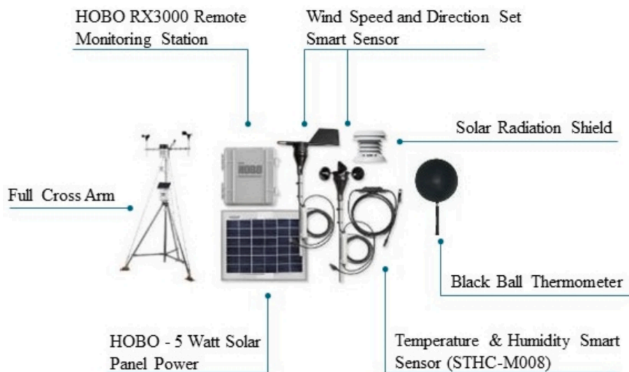
Fig. 3. Onset HOBO RX3000 Remote Monitoring Station.
