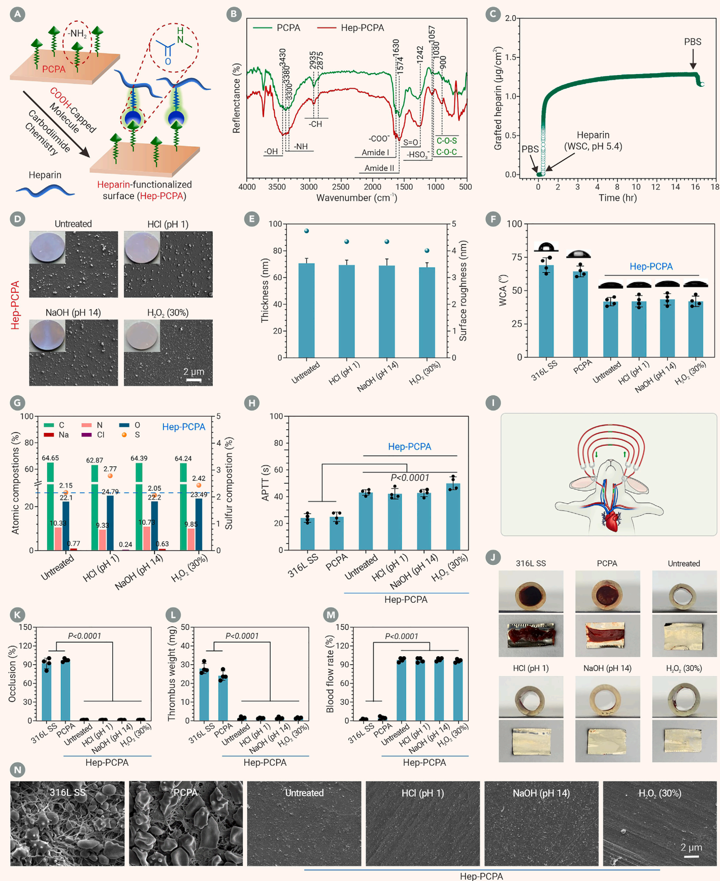
Figure 3. Secondary covalent immobilization of heparin onto PCPA coatings for developing durable antithrombotic surfaces (A) Schematic of heparin conjugation to PCPA-coated surfaces. (B) FTIR spectra of the PCPA-coated surfaces before and after heparin grafting. (C) Real-time analysis of the heparin grafting process by quartz crystal microbalance equipped with dissipation monitoring (QCM-D). (D) Macroscopic photos and SEM images of the Hep-PCPA-coated surfaces before and after treatment with HCl (pH 1), NaOH (pH 14),
