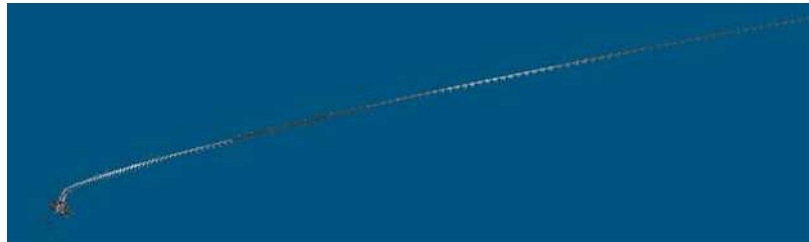
Fig. 1. An aerial view of a LiDAR scanning error model. The stilt house scanned is visible in the lower left and is considerably smaller than the error geometry proceeding upward and to the right.
