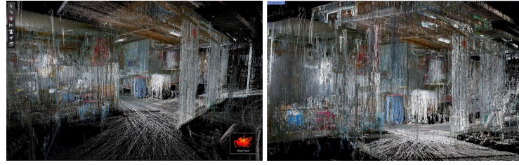
Fig. 2. A point cloud at original resolution in Cyclone 360 (left) and after decimation in Rhinoceros 3D (right).
