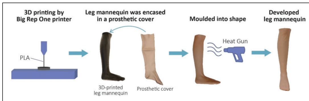
Figure 2. The development process of a 3D-printed leg mannequin
