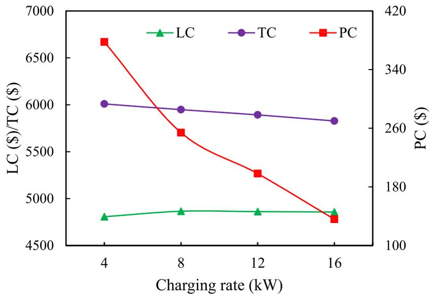
Fig. 7. Variations of the total operational cost, the total labor cost and the total penalty cost with the increase in charging rate.
