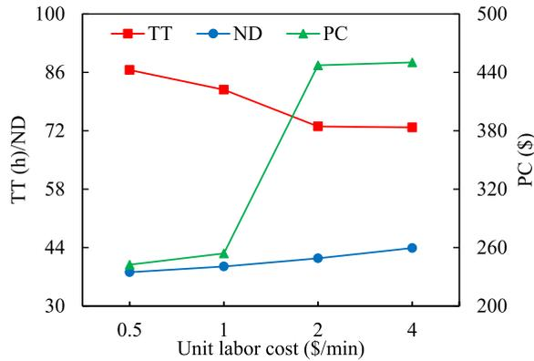
**Fig. 5.** Variations of the total penalty cost, the total working time of the drivers and the number of employed drivers with the increase of unit labor cost.
