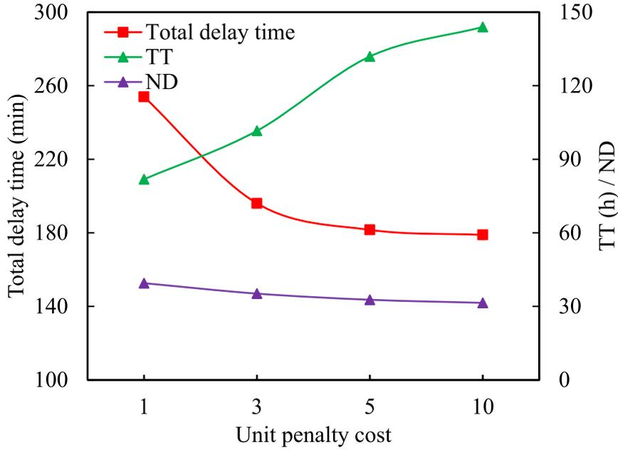
Fig. 6. Variations of the total delay time, the total working time of the drivers and the numbers of employed drivers with the increase in the penalty cost.
