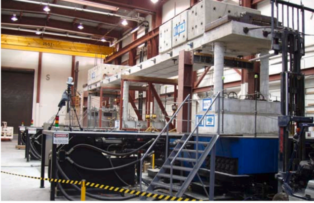
Fig. 2. The bridge model on the shaking table test [22].
