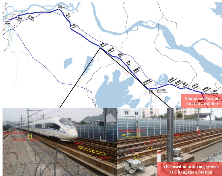
Fig. 12. AE-based rail turnout monitoring system at Changzhou station of Shanghai-Nanjing intercity rail line.
