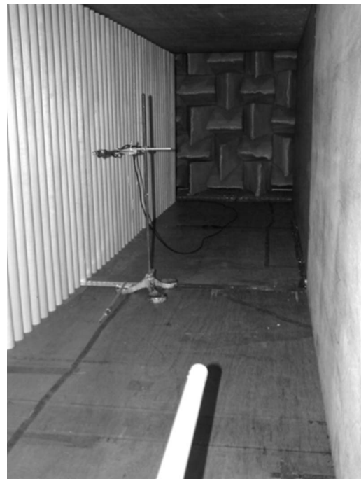
FIG. 5. An experimental setup in an anechoic chamber for measurement of sound propagation in a long enclosure with a roughening surface on the left vertical wall. Semicylindrical wooden rods of 0.015 m radius were taped securely on the wooden board. The rods were distributed pseudorandomly with a minimum center-to-center separation between two adjacent semicylinders b^* of 0.0525 m.
