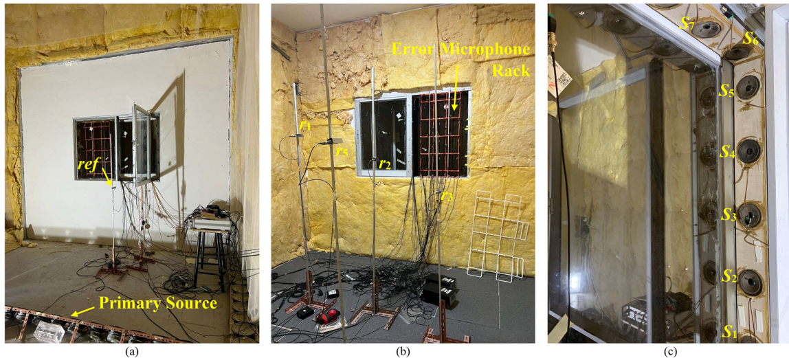
FIG. 3. (Color online) The physical experimental setup, showing (a) view of the plenum window from the source room, (b) plenum window viewed from the receiver room, and (c) close up of some secondary cancelling sources.
